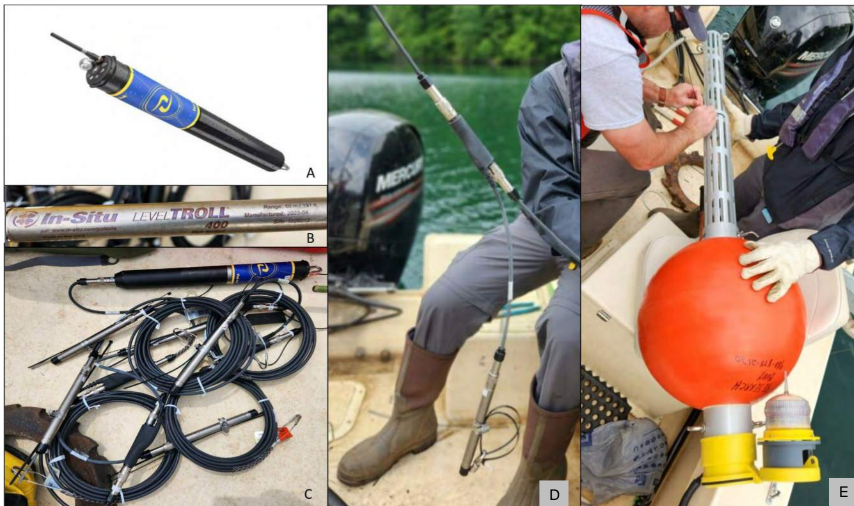
Figure 2. Water Quality Instrumentation: (A) VuLink device; (B) In-situ datalogger; (C) VuLink device and dataloggers on single continuous cable system; (D) Deploying stainless steel cable with dataloggers; (E) High visibility buoy with protective cage for VuLink device
