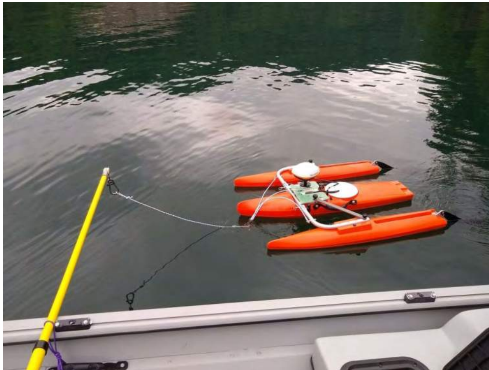
Figure 4-4. Teledyne RDI RiverRay ADCP and Trimaran
