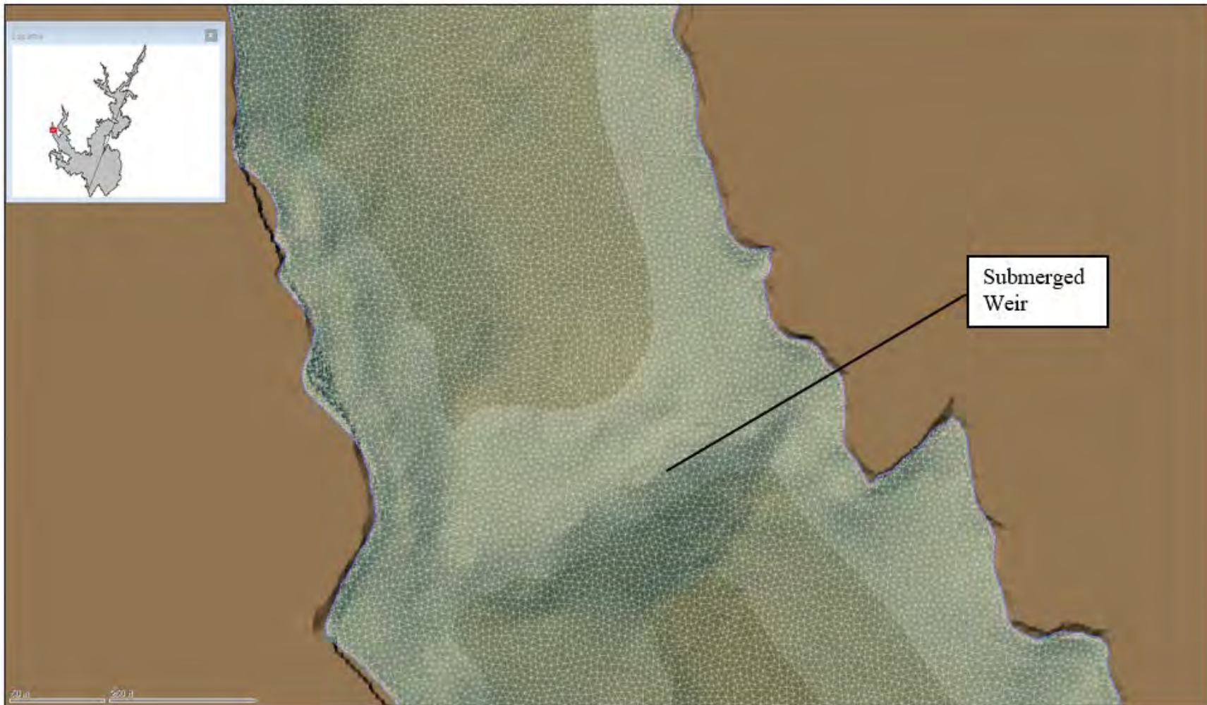
Figure 4-4. Example of 2-D Model Mesh Section
