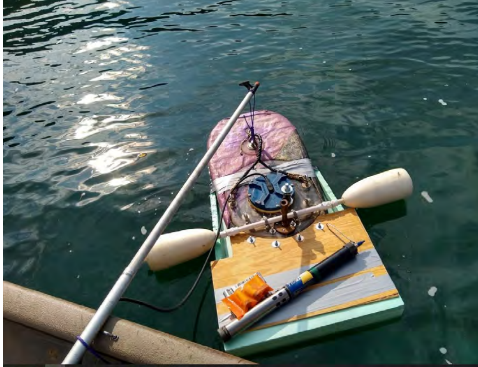
Figure 4-3. Teledyne RDI Workhorse Sentinel and Retrofitted Flotation Device
