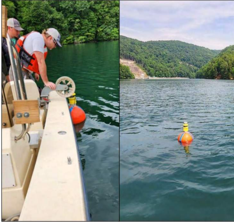
Figure 3. Instrumentation Deployment with Boat-mounted Winch (left) and Deployed Water Quality Monitoring Buoy and Datalogger Chain at Station 564.0 (right)
