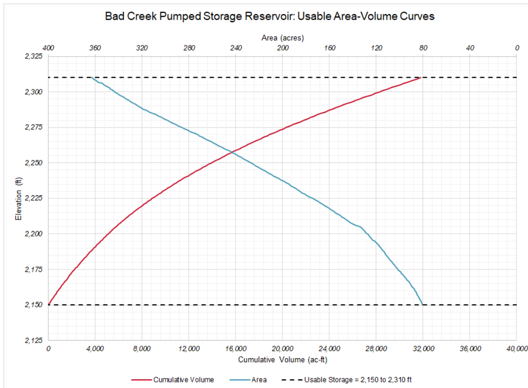
Figure B-1. Bad Creek Reservoir Total Area-Volume Curves
