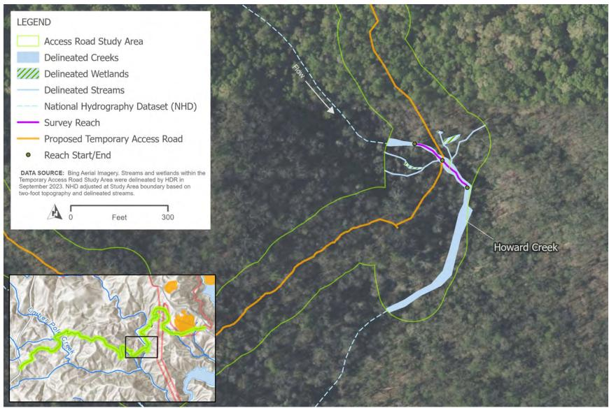
Figure 3. Stream 7 (Howard Creek) survey area and crossing of the proposed temporary access road
