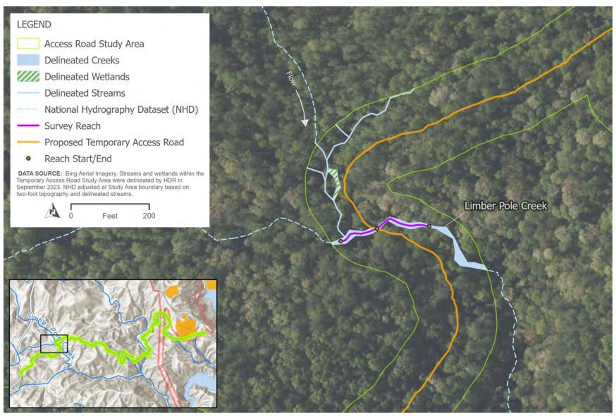
Figure 2. Stream 1 (Limber Pole Creek) survey area and crossing of the proposed temporary access road
