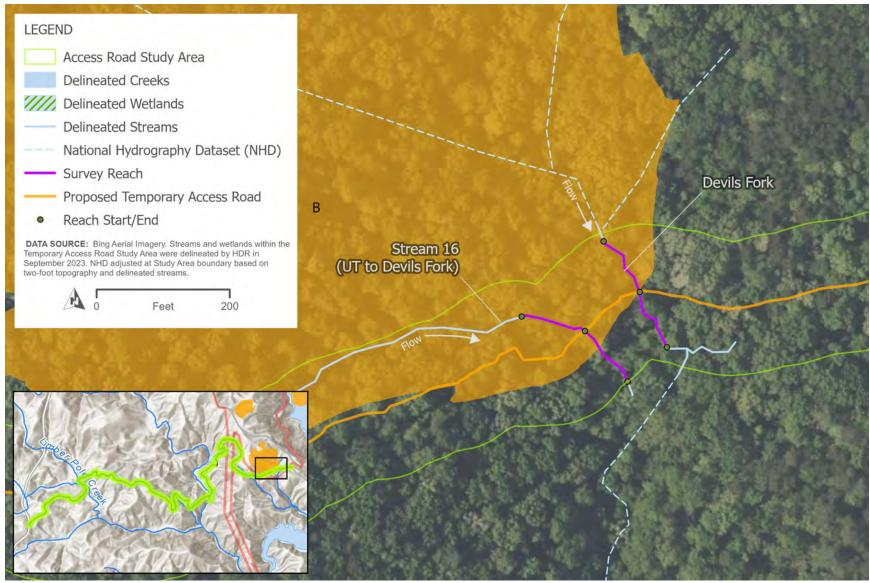
Figure 6. Stream 16 and Stream 17 (Devils Fork) survey area and crossing of the proposed temporary access road
