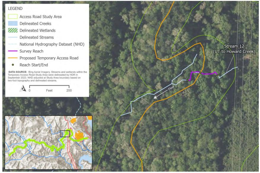
Figure 4. Stream 12 survey area and crossing of the proposed temporary access road
